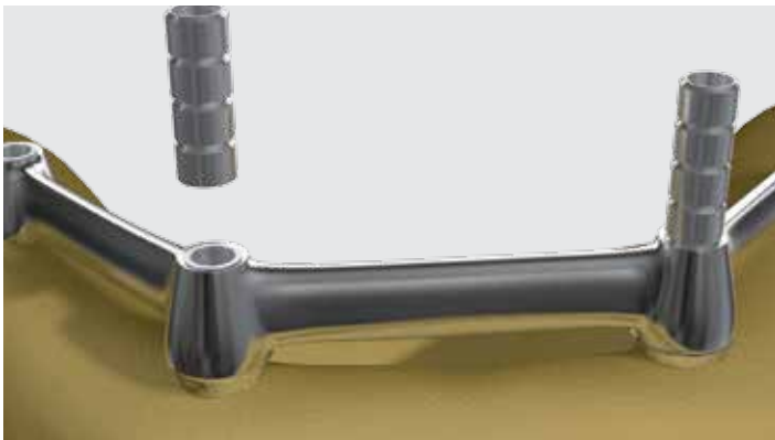
24 In the last step, shorten the Multi-Unit Caps titanium (Ref. 3111) that stick out.
